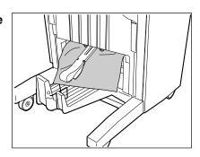
6 Open the exit cover of the saddle stitcher and remove any misfed paper.
